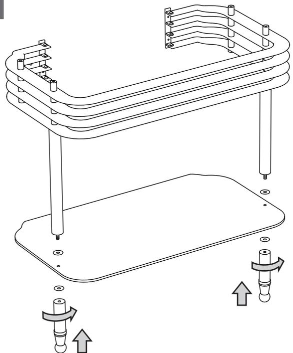
**3** Temporarily place the stand in the desired position. Once in place, mark all the fixing points on the wall and mark the footprint of the legs onto the floor to confirm the floor fixing position.
