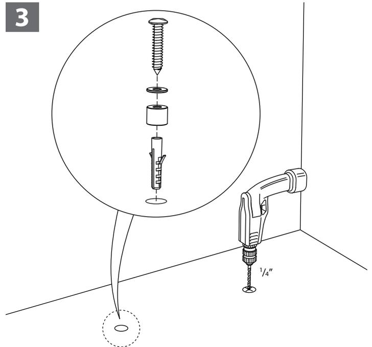
Drill 2 holes ( $\frac{1}{4}$ " in diameter) in the center of the floor fixing positions, then fix the floor nipples onto the floor as shown.
