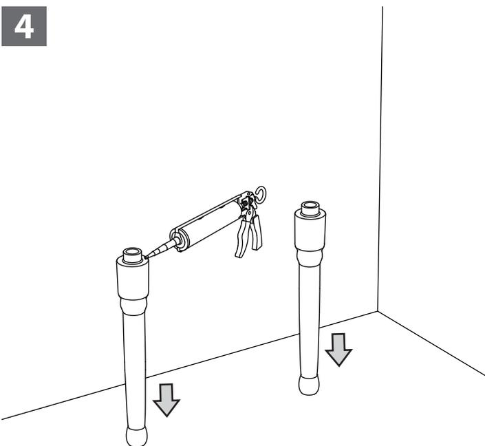
Carefully apply silicone on the top of the legs and then locate the legs over the floor nipples.
