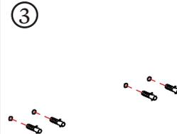
Insert the wall anchors into the drilled holes.
