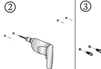
Using a 6mm or 1/4" drill bit, drill holes in the marked positions.
