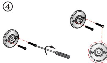
Use the flat-head screwdriver and the stainless steel screws to secure the base to the wall. Please ensure that the slot on the screw heads are horizontal.
