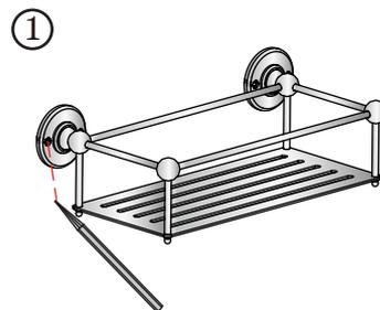
Determine the final installation position, mark the mounting hole positions in pencil.
