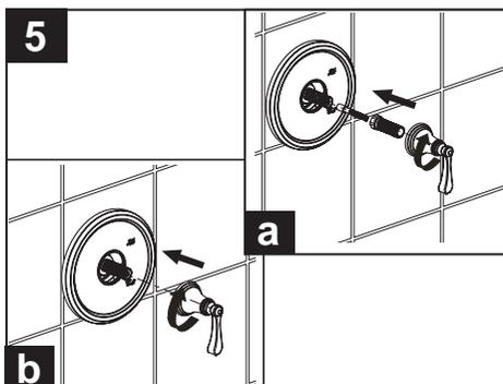
a.) Add the threaded nipple and pressure balance stem extensions.
