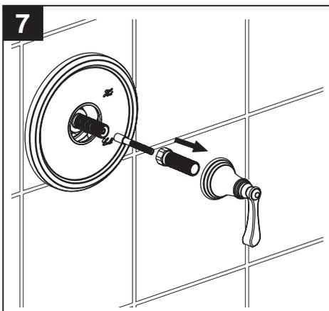
Remove the handle assembly and nipple and stem extensions.
