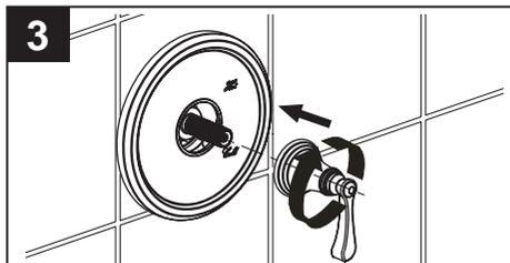
Place the handle assembly on the valve and rotate clockwise securing the handle assembly and escutcheon to the wall and engaging the stem.
