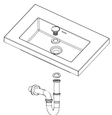
NOTE: The basins are not come with pre-drilled tap holes, the semi-punched tap hole is recessed at the back side of the top hole position.
