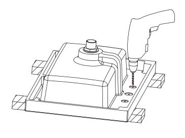
Place the basin upside down on a stand. Add a layer of protection between the stand and basin to avoid surface damage or scratching. Aim the Ø3mm drill bit at pilot hole at the back side of the basin, then drill through the pilot hole.
