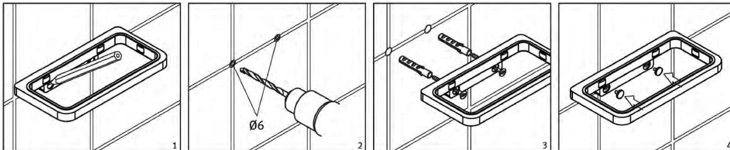
Check that there are no concealed water pipes or electrical cables before drilling into the wall. The product should be installed by a professional, following the recommended installation. Before beginning installation, check for any damage that may have occurred during transport.
