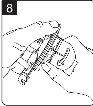
8 Remove the flapper from the flush valve by pulling up the frame of flapper one side at a time.
