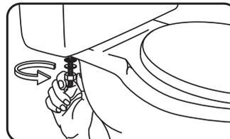
Then place the tank back on the bowl so that the tank-to-bowl gasket fits evenly. Level the tank. Under the bowl, attach a rubber washer, a metal washer and a metal hex nut. Tighten the hex nuts under the bowl evenly until the tank is stable and doesn't rock. **DO NOT OVERTIGHTEN** or the tank or bowl could break.
