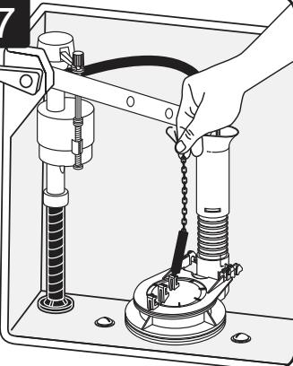
Connect the flapper chain to the tank lever. Allow for 1/2" of slack in the chain when the flapper is closed.
