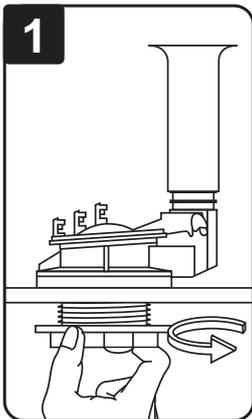
**1** Before installing the flush valve in the tank, remove the tank-to-bowl gasket and nut from the bottom of the threads of the new flush valve. Position the overflow pipe toward the back of the tank but not over the bolt holes. Thread large nut onto the threads. Hand tighten only. **DO NOT OVERTIGHTEN** or tank may crack.
