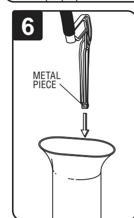
The refill clip must be attached to the top of the overflow pipe. Place metal piece of refill clip against the outside edge of the pipe then press against the overflow pipe. When the inside prong clears the top edge of the pipe, push the clip down. Attach the refill hose to the nipple of the refill clip and the other end to the nipple of the fill valve. You many need to trim the rubber hose.
