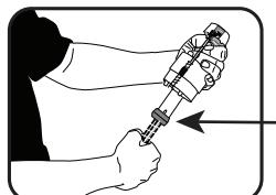
Position fill valve in tank, but do not fully install yet. Top of fill valve MUST be set 3" above overflow pipe. This will automatically place **CRITICAL LEVEL MARK / C.L. Mark**, 1" above the top of overflow pipe. Remove fill valve from tank to adjust height.
