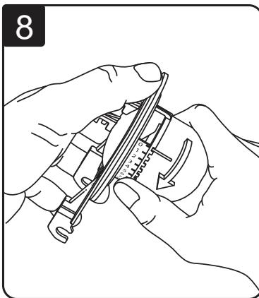
Remove the flapper from the flush valve by pulling up the frame of the flapper one side at a time.
