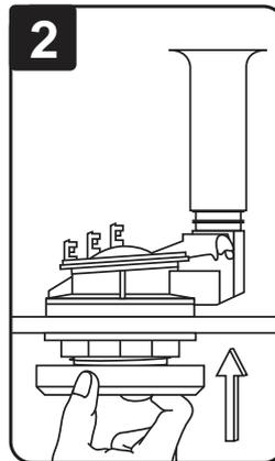
**2** Slide new tank-to-bowl gasket over the nut with the narrow side facing down. Gasket should cover the nut completely.
