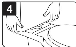
**4** Optional: Before replacing the tank on the bowl, place a metal washer and hex nut onto the bolt under the tank and hand tighten until snug.
