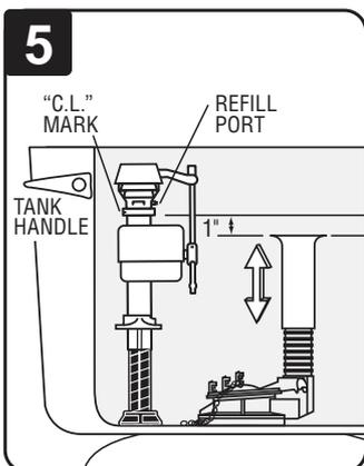
**5** When installed, the top of the overflow pipe of the flush valve must be at least 1" below the C.L. mark of the fill valve.
