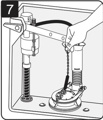
7 Connect the flapper chain to the tank lever. Allow for 1/2" of slack in the chain when the flapper is closed.
