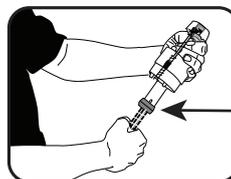
Position fill valve in tank, but do not fully install yet. Top of fill valve **MUST** be set 3" above overflow pipe. This will automatically place **CRITICAL LEVEL MARK / C.L. Mark**, 1" above the top of overflow pipe. Remove fill valve from tank to adjust height.
