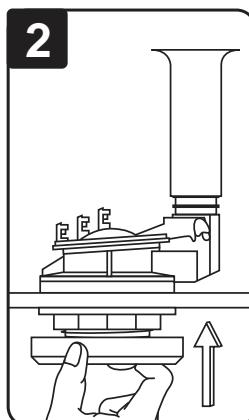
Slide new tank-to-bowl gasket over the nut with the narrow side facing down. Gasket should cover the nut completely.
