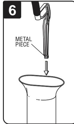
**6** The refill clip must be attached to the top of the overflow pipe. Place metal piece of refill clip against the outside edge of the pipe then press against the overflow pipe. When the inside prong clears the top edge of the pipe, push the clip down. Attach the refill hose to the nipple of the refill clip and the other end to the nipple of the fill valve. You may need to trim the rubber hose.
