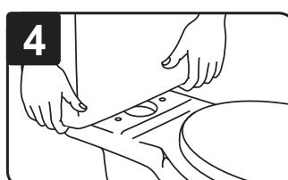
Optional: Before replacing the tank on the bowl, place a metal washer and hex nut onto the bolt under the tank and hand tighten until snug.
