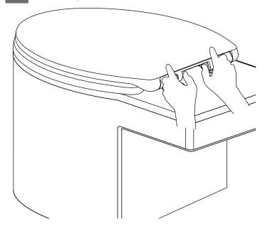
Open the seat to the vertical position, then lift the seat straight up with one hand.
