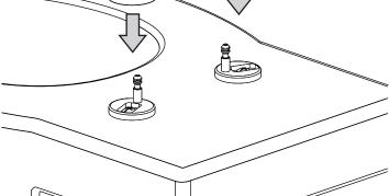
When mounting the seat make sure the posts align with the holes in the back of the seat. Carefully lower the seat back into place (a "click" will heard).
