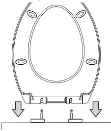
To remove the seat, press the quick-release button (you should hear a "click")
