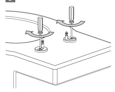
NOTE: Only install and dismantle the seat and cover at an angle of 90±5°. Failure to do this will result in damage to the seat and cover.
