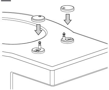
When mounting the seat make sure the posts align with the holes in the back of the seat. Carefully lower the seat back into place (a "click" will heard).
