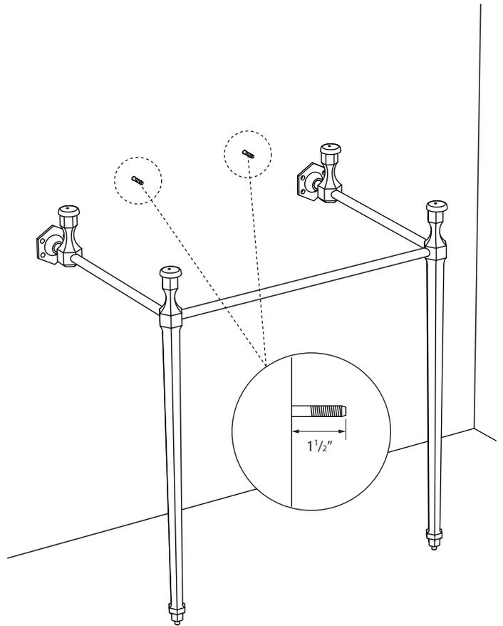
**12** Position the basin on the frame so the hanger bolts extend through the fixing holes. Secure the basin using cap nuts and washers, **DO NOT OVERTIGHTEN!**
