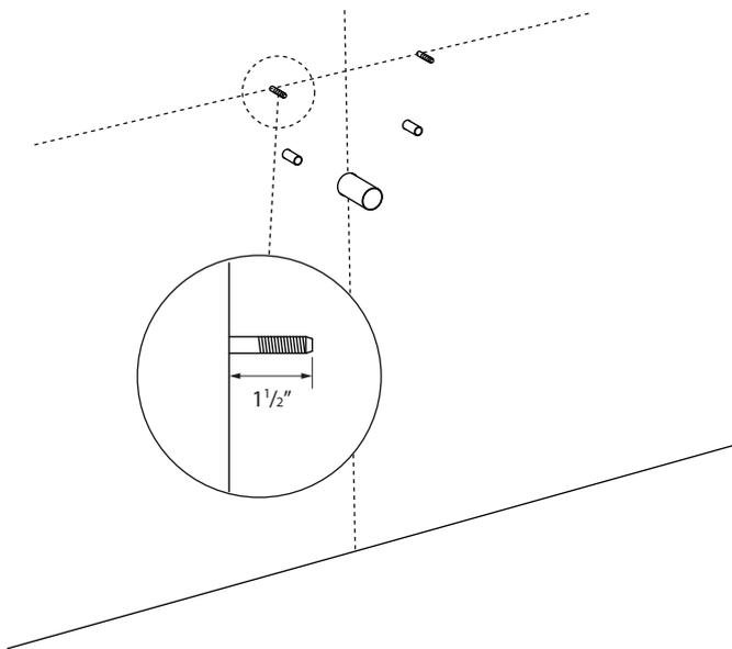
**7** Position the basin on the hanger bolts through the fixing holes.
