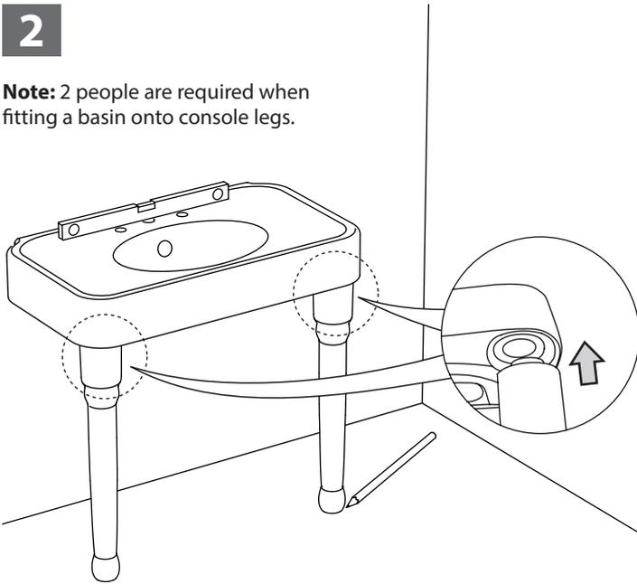
Temporarily mount the basin onto the 2 legs and locate against the wall in the desired position. Once in place, mark the footprint of the leg base onto the floor to confirm the floor fixing position.
