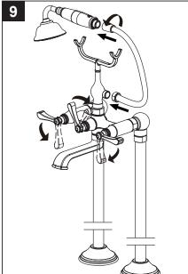
Attach hose to spout and handheld shower. Turn on the water supply to test the hot, cold and diverter water flow.
