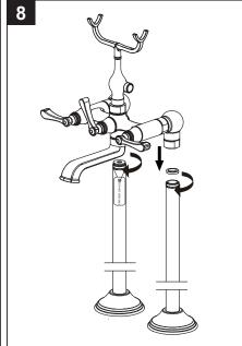
Mount valve body on the riser pipe
