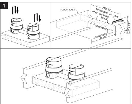
Adequate floor support is required. The WOOD SUPPORT must be a minimum of 2" (51mm) thick by 10" (254mm) wide. Wood support must be located within the MIN. and MAX. arrows that are marked on the plaster guard. Use 4 screws to install and fix the mounting base to the wood support board. Use level from bottom on both directions to make sure wood support board is flat. Secure wood support to floor joists.
