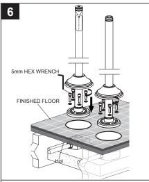
Before final installation, check that all sealing surfaces are clean. Install the mounting adapters onto the mounting base. Install the mounting screws and washers through the mounting plate. And into the mounting base. Do not tighten. Rotate the tub filler right or left to align with tub. Tighten mounting
