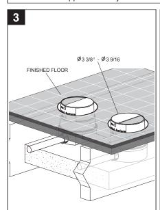
Assure the valves are centered in holes that are 3-1/4" to 3-5/8" diameter. This is required to allow mounting base to be installed properly.
