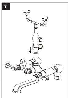
Attach handshower yoke to valve body. Assure the washer is in place.
