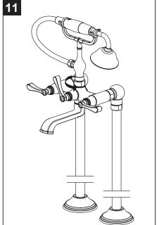
To adjust the handshower yoke to reverse direction, unscrew the nut and rotate the yoke by 180 degree and then tighten the nut.
