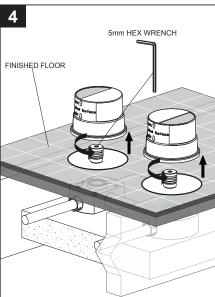
Turn water supply off. Remove the plaster guards and the test plugs with the supplied hex wrench.
