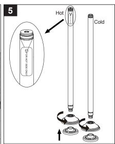
Slide escutcheons onto riser pipe. Thread hot and cold riser pipes into the appropriate side of the mounting base making sure the hot riser is attached to the hot water supply as noted in the image above.
