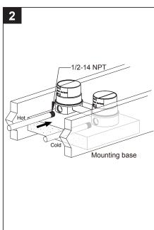
Thread and securely tighten 1/2" male NPT hot and cold supply lines into the mounting base. Make sure the hot line is installed on the left side of the mounting base when facing the mounting base from the front of where the floor tub filler will fill the bathtub.
