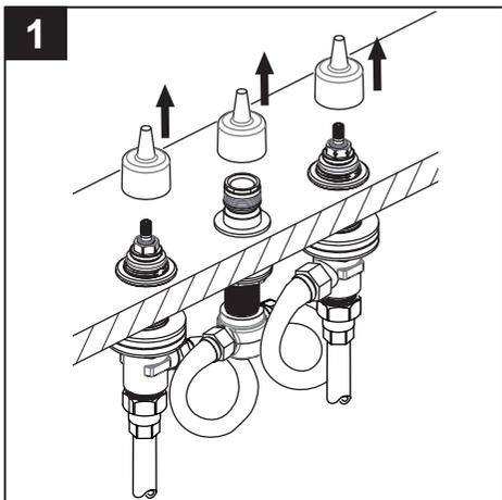
Remove the mud guards from the spout nipple assembly, the hot and cold valves.
