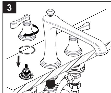
Place the "O" ring over the cold valve. Align the handle and escutcheon assembly into the valve. Secure the assembly by turning the escutcheon clockwise. Repeat for hot valve.
