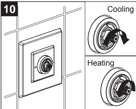
If the temperature in #8 was less than 100° turn the temperature limit ring to the left. If the temperature was more than 100° turn the temperature limit ring to the right. Reinstall the handle and escutcheon.
