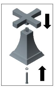
2. Take out the screw and lock washer with a Phillips screwdriver
