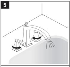
Remove the aerator with the supplied key. Turn the faucet handles on full for one minute to flush debris.
