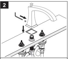
Place the spout washer under the spout and install spout on spout nipple assembly. Be sure the spout is firmly resting on the deck and secure the spout. Secure the spout with the setscrew.
