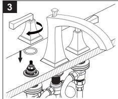
Place the "O" ring over the cold valve. Align the handle and place the handle and escutcheon assembly into the valve. Secure the assembly by turning the escutcheon clockwise. Repeat for hot valve.
