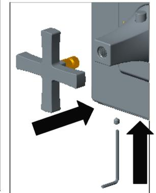
1. Remove the set screw with an Allen wrench (2.5mm)
