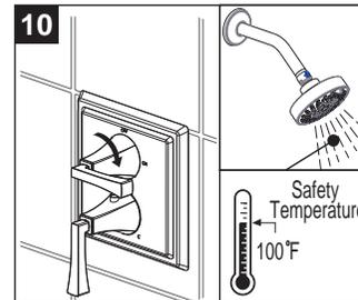
Turn on the water supply, with the temperature control handle in the default position, measure the temperature of the water. If the temperature is 100°F, go to step #14, if not go to step #11.
