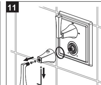
Turn off the water supply. Remove temperature control handle and escutcheon.
