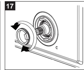
Rotate the inner white temperature range control ring to adjust temperature. Rotate clockwise to reduce temperature while rotate counterclockwise to increase temperature.
