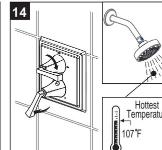
The valve maximum temperature is set at 107°F. Should your customer like to change this go to step #15. If not go to step #20.
