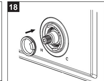
Reinstall the inner white temperature range control ring.
