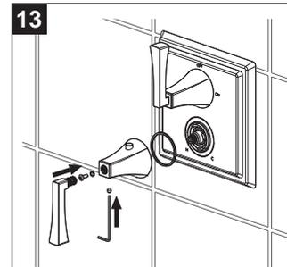
Reinstall the temperature control handle and escutcheon making sure the temperature override button is on top and the handle is set at 6 o'clock.
