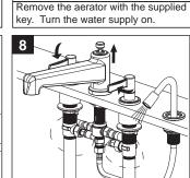
Leaving the water on, pull the hose to its farthest extension and point it into the tub. Pull the diverter knob to its top position. Flush the debris for one minute. Turn off the valves.
