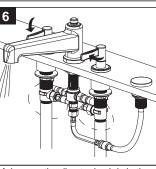
Make sure the diverter knob is in the down position. Turn the faucet handles on full for one minute to flush debris.
