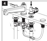
Align the handle and place the handle and escutcheon assembly into the valve. Secure the assembly by turning the escutcheon clockwise. Repeat for hot valve.
