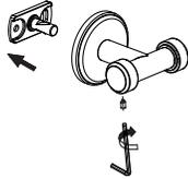
Loosen the set screw and slide out the fixed mounting bracket
