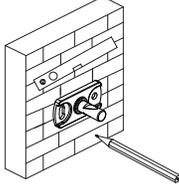
Mark drill holes in desired location.
