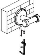
Place accessory on the mounting bracket. Secure it to the wall using the bottom set screw.
