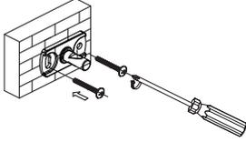
Place the mounting bracket over the wall anchors. Secure it to the wall using the supplied screws.
