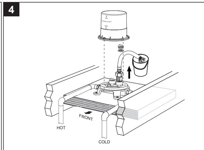
Finish all Hot and Cold supply connections to the MANIFOLD MOUNTING BASE. Loosen the two PLASTER GUARD SCREWS and remove the PLASTER GUARD. Make sure the two TEST PLUGS are tight, but do not over tighten. Turn on water supplies and test for leaks. Turn off water supplies. Replace PLASTER GUARD and attach with SCREWS.
