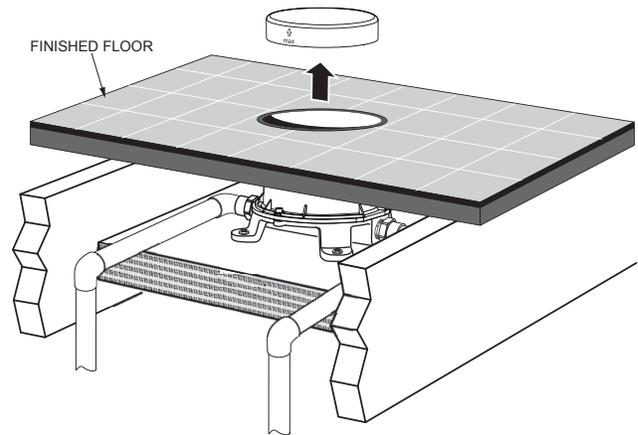
When you are ready to install the TUB FILLER cut the exposed part of the PLASTER GUARD flush with the finished floor. Be careful not to damage the floor.
