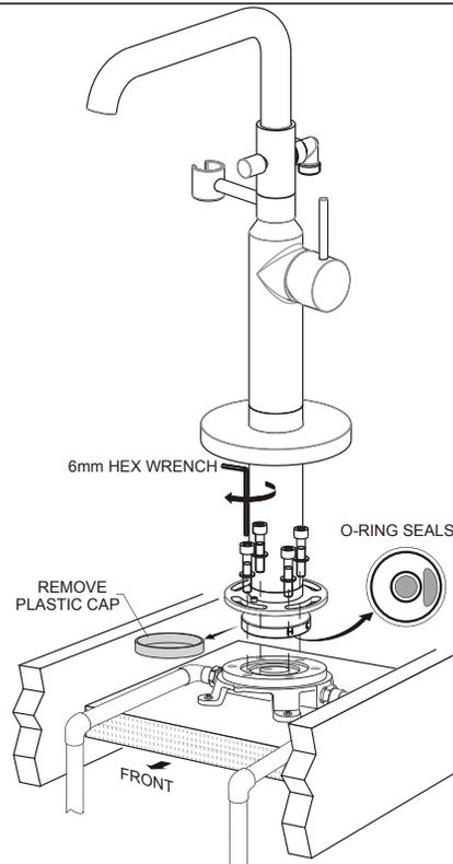
Remove PLASTIC CAP from bottom of the TUB FILLER. Before final installation, check that all sealing surfaces are clean and that the two O-RINGS are installed in the MOUNTING ADAPTER. Install the MOUNTING ADAPTER into the MANIFOLD MOUNTING BASE. Install the four MOUNTING SCREWS and WASHERS through the MOUNTING PLATE and into the MANIFOLD MOUNTING BASE. Do not tighten. Rotate the TUB FILLER right or left to align with Tub. Tighten MOUNTING SCREWS supplied with 6mm Hex Wrench to secure TUB FILLER.
