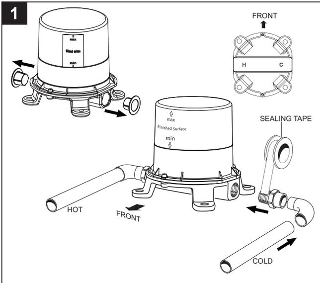
Sweat together Hot and Cold Supply assemblies. Apply sealing tape to threaded connections. With the maximum and minimum measurement in front, the hot supply is to be installed on the left inlet and the cold on the right as shown in the image above.
