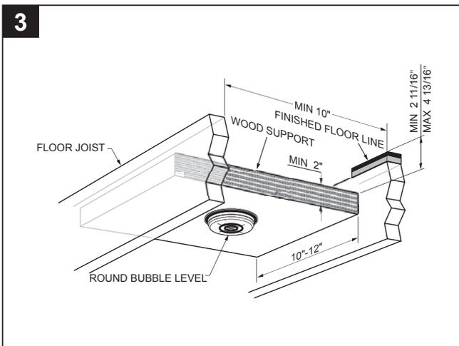
Adequate floor support is required. The WOOD SUPPORT must be a minimum of 2" (51mm) thick by 10" (254mm) wide. 2x6 lumber is NOT adequate for this application. WOOD SUPPORT must be located within the MIN. and MAX. arrows that are marked on the front of the PLASTER GUARD.
