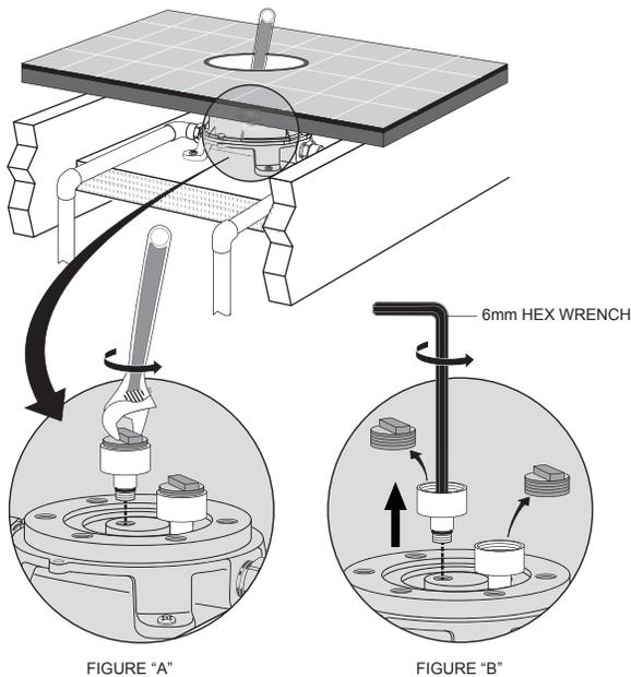
Turn off water supplies. With a wrench remove the center TEST PLUG as shown in Figure A. If the TEST PLUGS cannot be removed in one piece as shown in Figure A, the lower half will have to be removed using the supplied 6mm Hex Wrench as show in Figure B. Repeat step for the second TEST PLUG.
