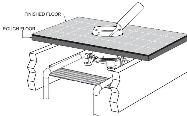
Complete the installation of the Finished Floor. Tile as close to the PLASTER GUARD as possible. Caulk between Finished Floor and PLASTER GUARD.
