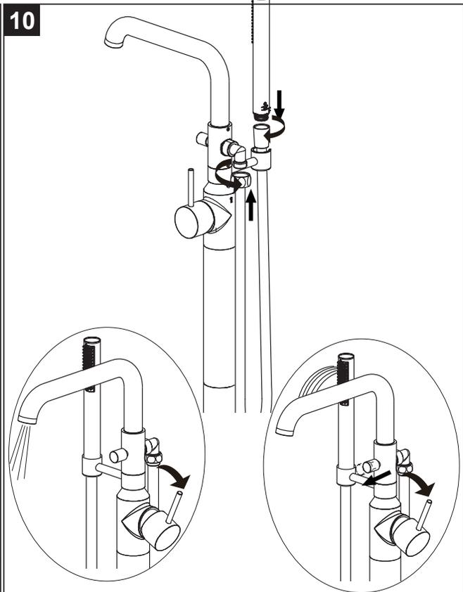
Attach hose to spout and handheld shower. Once hand shower is attached turn on TUB FILLER and test the diverter
