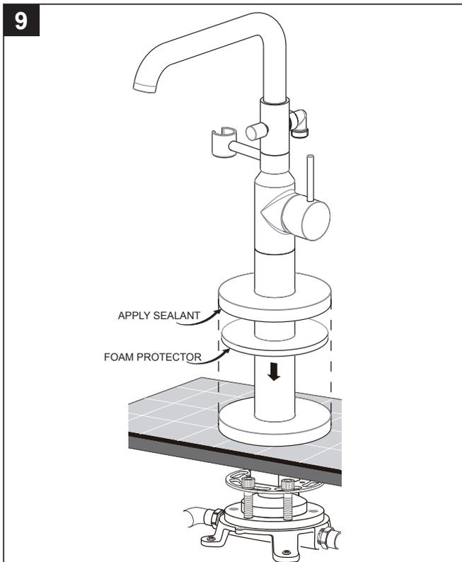
Turn on water supplies and check all connections for leaks. Check MANIFOLD connections for leaks. Remove foam protector and apply sealant to under side edge on ESCUTCHEON . Slide ESCUTCHEON down to finish floor. Press into place. Clean up excess sealant.
