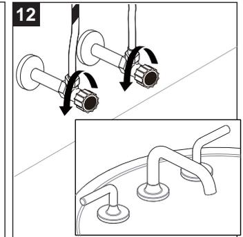
12 Turn on angle stops and check all connections for leaks.
