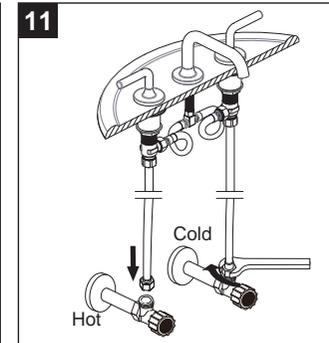
11 Attach customer-supplied water supply lines.
