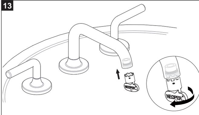
13 Remove aerator with key and flush out debris. Reinstall aerator and save aerator key for homeowner.
