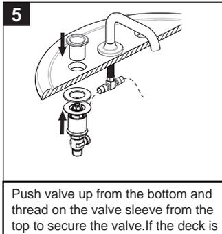
Push valve up from the bottom and thread on the valve sleeve from the top to secure the valve. If the deck is less than 1 3/8" thick use the supplied spacer. If the deck is thicker than 1 3/8" do not use the spacer.
