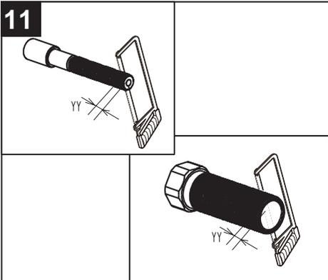
Cut stem and nipple extensions the amount noted in step # 9. (Never cut the stem and nipple while still on the valve. This may damage the valve.)
