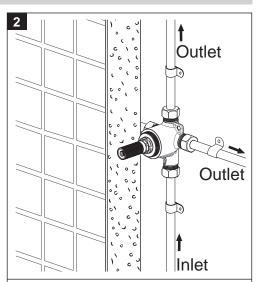
Install the valve with proper fitting or use mounting holes on valve. Support as noted in image. Turn on water supply and inspect for leaks.
