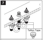
Apply teflon tape to the hot and cold valve inlets on the spout nipple-diverter assembly and attach the hot and cold flex lines.
