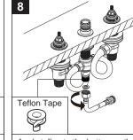
Apply teflon to the bottom outlet on the spout nipple-diverter assembly and attach the rough hand shower hose with washer.
