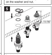
Push the hot and cold valves up from the bottom and thread on the valve nuts from the top to secure the valves.
