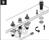
Slide the hand shower hose guide nipple into the appropriate hole and secure by threading on the nut and washer. For optimum hand shower usage it should be located no father than 24" from the spout.
