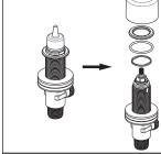
Remove the mud guards from the hot and cold valves.
