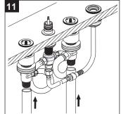
Connect valve body to water supplies using the proper fittings.
