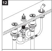
Turn on water supply and check for leaks.
