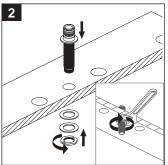
Slide the spout nipple down into the spout hole and secure by threading on the washer and nut.
