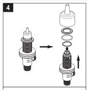
Remove the mud guards from the hot and cold valves.
