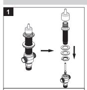
Remove the mud guard from the spout nipple-diverter assembly and unthread the diverter assembly.
