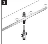
Re-attach the diverter assembly to the spout nipple.
