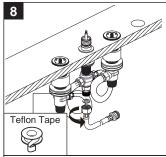
Apply teflon to the bottom outlet on the spout nipple-diverter assembly and attach the rough hand shower hose with washer.
