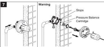
Connect valve body to water supplies using the proper fittings.
