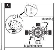
Using mounting holes secure the valve making sure the "UP" label outlet is on top.
