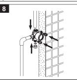
Connect the valve body to the shower outlet with the proper fitting. Note: it is suggested that you anchor all water lines and reinstall stops and cap.
