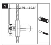
This valve is designed to fit into a wall that is 2-7/8" to 3-7/8" from finished wall to the back of the valve. Extensions are available separately if necessary.
