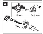
Align the pins on the bottom of the cartridge and push the cartridge into the valve. Make sure the cartridge is firmly installed into the valve body. Reinstall stem assembly with mud guard.
