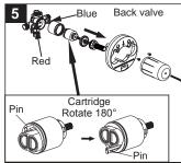
Remove the cartridge and stem assembly. Notice that the pin is at the top. Rotate the cartridge 180°. The pin should be on the bottom.
