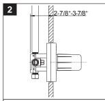
Turn off the water supplies.Install the valve so the finished wall will fit between the markers on the mud guard.
