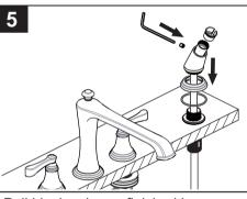
Pull black nylon or finished hose through the hand shower nipple bracket. Slide the hand shower "O" ring, bracket and hose guide over the hose. Secure the assembly with the setscrew. Note, make sure the hose does not slip under the deck.
