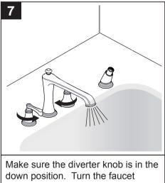
down position. Turn the faucet handles on full for one minute to flush debris.
