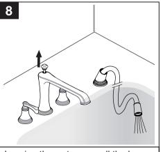
Leaving the water on, pull the hose to its farthest extension and point it into the tub. Pull the diverter knob to its top position. Flush the debris fro one minute. Turn off the valves.
