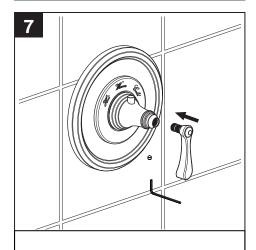
Slide handle into escutcheon and secure with set screw.
