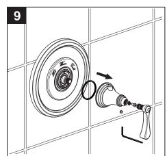
Turn off the water supply. Remove handle and escutcheon.
