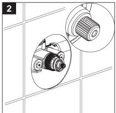
NOTE: Make sure the hole in the stem is facing straight up. (This sets the valve at 100°).
