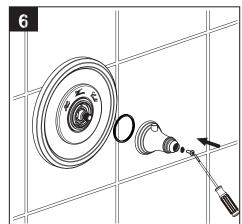
Slide on escutcheon engaging the stem making sure the temperature override button facing straight up. Secure with screw.
