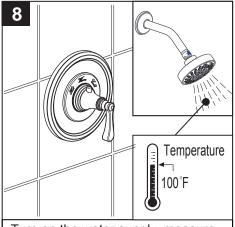
Turn on the water supply, measure the temperature of water. If the temperature is 100°F,go to step #9, if not go to step #11.
