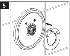
Slide on top plate on the finished sleeve. If the top plate does not engage the finished sleeve an extension kit is necessary. Please contact your Crosswater London dealer.
