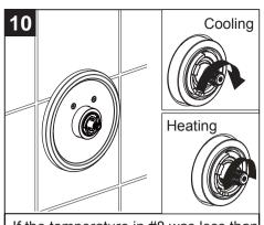
If the temperature in #8 was less than 100° turn the temperature limit ring to the left. If the temperature was more than 100° turn the temperature limit ring to the right. Reinstall the handle and escutcheon.
