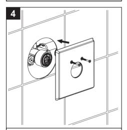
Install escutcheon with 2 screws. Do not overtighten the screws.
