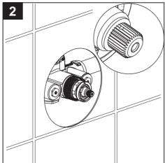
NOTE: Make sure the hole in the stem is facing straight up. (This sets the valve at 100°).
