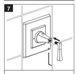
Slide handle into escutcheon and secure with set screw.
