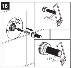
Cut stem and nipple the amount noted in step # 14. (Never cut the stem and nipple while still on the valve. This may damage the valve.)
