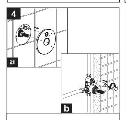
Remove escutcheon and diverter sleeve, stem and button.
