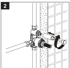
Install diverter sleeve, stem and button on to the valve.
