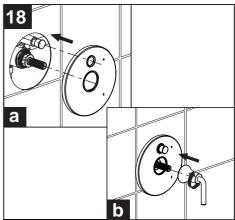
Place escutcheon on valve. Thread on handle assembly to secure escutcheon.
