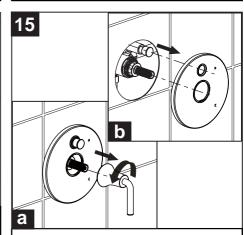
Remove the handle and escutcheon assembly, the plate, stem and nipple.
