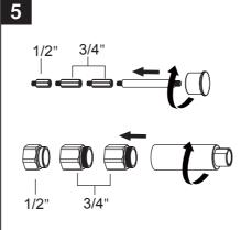
Install the appropriate diverter stem and sleeve extensions supplied with the trim to allow easy access to the diverter button.
