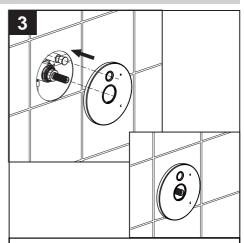
Carefully slide escutchen on valve. If diverter knob is accessible, go to step #13. If not continue to step #4.
