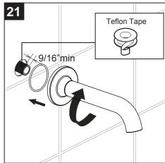
Apply teflon tape to the tub spout nipple and thread on wall tub spout.
