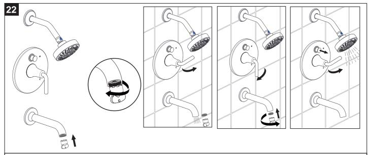
Remove tub spout flow guide with key and flush out debris. Reinstall flow guide and save key for homeowner.
