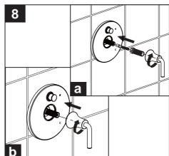
a.) Add the threaded nipple and pressure balance stem extensions.
