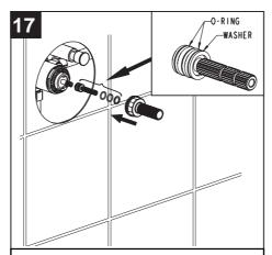
Re-install the trimmed stem and nipple on the valve.
