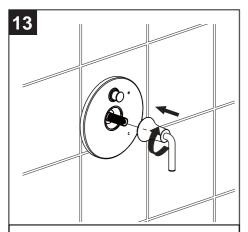
Place handle assembly on valve and rotate clockwise to secure escutcheon.
