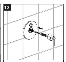
Re - install the nipple and stem extensions. Then, go to step #19.
