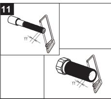
Cut stem and nipple extensions the amount noted in step # 9. (Never cut the stem and nipple while still on the valve. This may damage the valve.)
