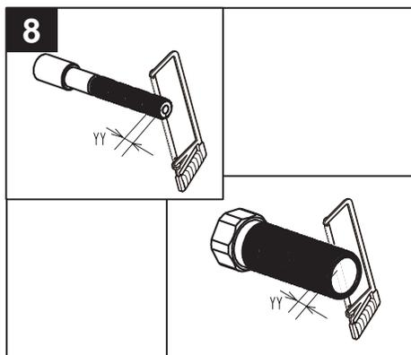
Cut stem and nipple extensions the amount noted in step # 6. (Never cut the stem and nipple while still on the valve. This may damage the valve.)
