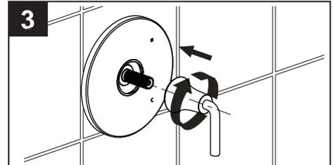
Place the handle assembly on the valve and rotate clockwise securing the handle assembly and escutcheon to the wall and engaging the stem.
