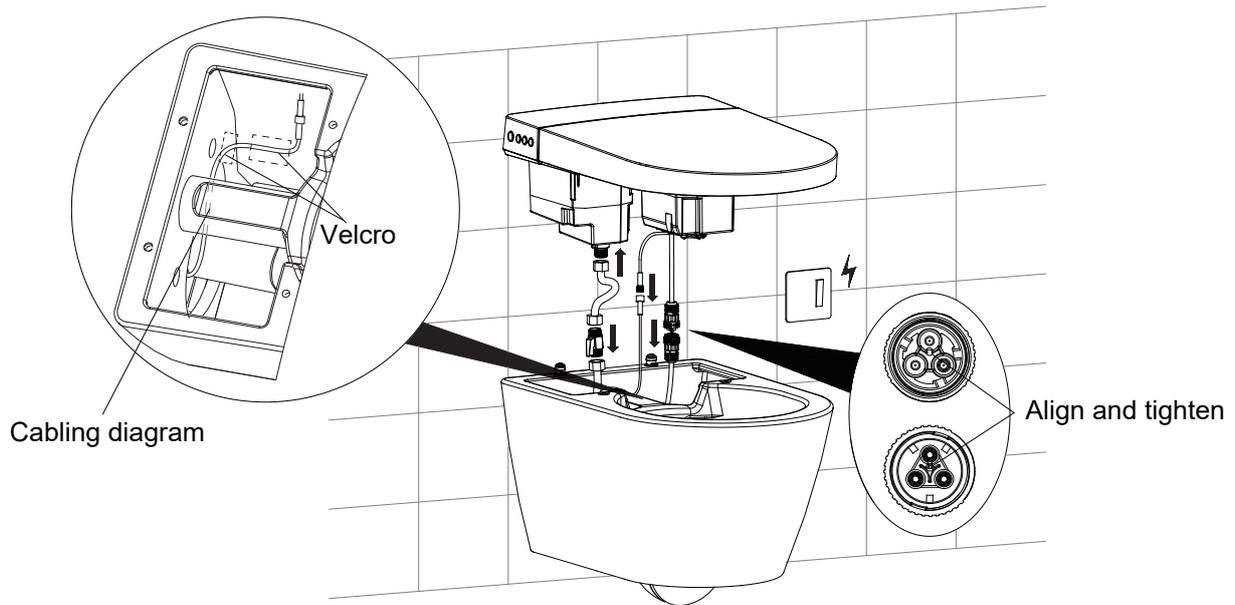
21. Position the seat and check the alignment.
