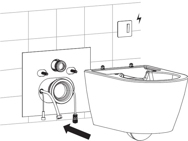
15. Fit the water supply hose, off-seat auto flushing cable and power cord through the toilet.
