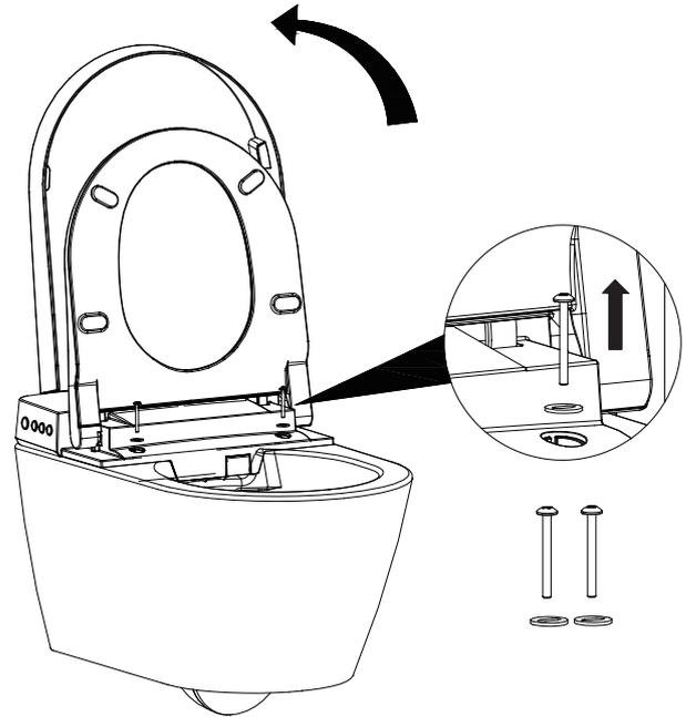
3. Close the seat, and remove it from the toilet. Gently put it on a clean cardboard to avoid any damage.
