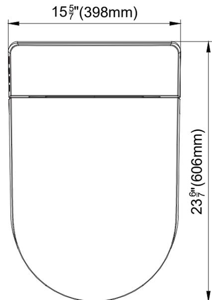
The above dimension is based on toilet being installed with Ressa in wall carrier US-RS200-TC, and with minimum adjustment.
