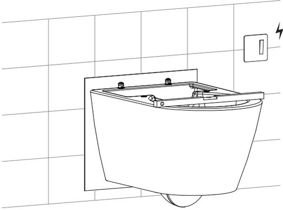
17. Fix the toilet onto the wall.
