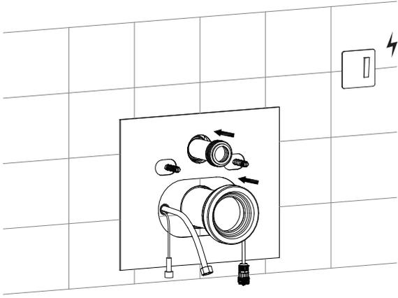
13. Apply silicone oil on the flush pipe and discharge pipe.
