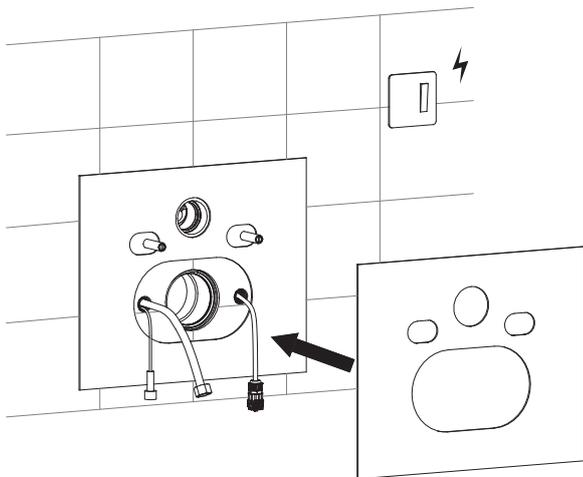
11. Remove the protective sleeve on bolts. Apply silicone oil on the in-wall flush pipe and drain pipe orifice.
