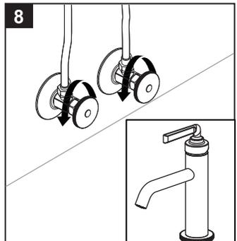
Turn on angle stops and check all connections for leaks.
