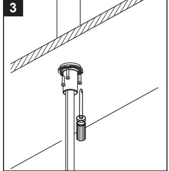
Use a screwdriver to tighten the lock nut.
