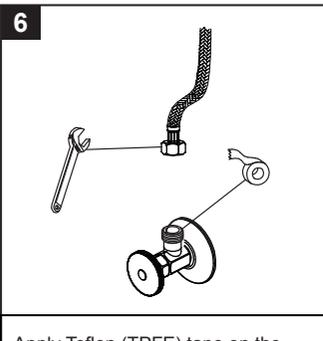
Apply Teflon (TPFE) tape on the shut off valves. Thread the tape in acounter-clockwise direction.
