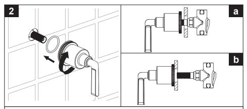
Place the "O" ring over the stem and nipple assembly. Align the handle and place the handle and escutcheon assembly into the valve. Secure the assembly by turning the escutcheon clockwise.
