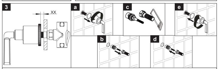
Measure and note the distance 'XX' between the finished wall and the bottom of the escutcheon.
