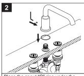
Place the spout "O" ring under the spout and install spout on spout nipple assembly. Be sure the spout is firmly resting on the deck and secure the spout. Secure the spout with the setscrew.
