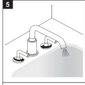
Remove the aerator with key. Turn the faucet handles on full for one minute to flush debris.
