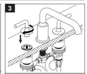
Align the handle and place the handle and escutcheon assembly into the valve. Secure the assembly by turning the escutcheon clockwise. Repeat for hot valve.
