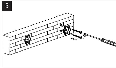
Place the mounting brackets over the wall anchors. Secure them to the wall using the supplied screws.
