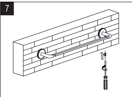
Place towel bar assembly on the mounting brackets. Secure it to the wall using the bottom set screws.
