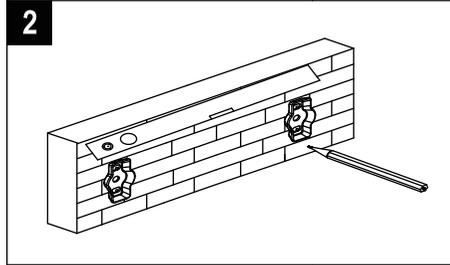
Align brackets and mark drill holes in desired location.
