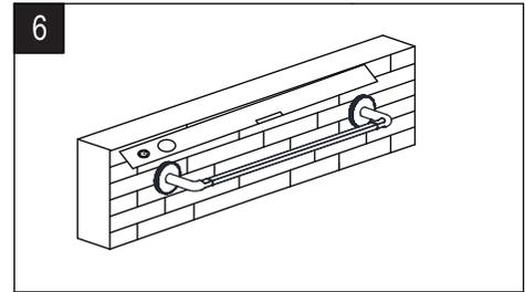
Temporarily place the towel bar on the mounting brackets to check alignment. If necessary, loosen the screws and realign the mounting brackets.
