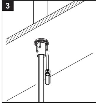
Use a screwdriver to tighten the lock nut.
