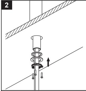
Install the washer and gasket onto the threaded tube.
