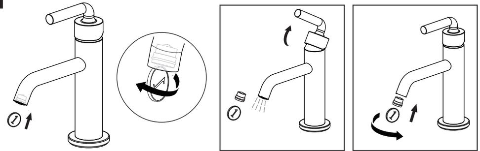
Remove aerator with coin and flush out debris.
