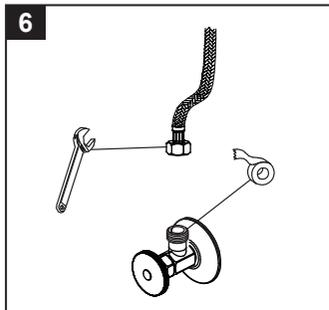
Apply Teflon (TPFE) tape on the shut off valves. Thread the tape in acounter-clockwise direction.
